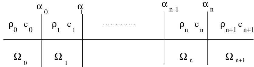
FIGURE 1. Cracks \alpha_k separating elastic media \Omega_k and \Omega_{k+1} . The physical parameters are the density \rho_k and the sound speed c_k .
